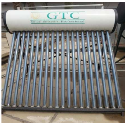
Fig 3. The experimental evacuated tube solar collector
