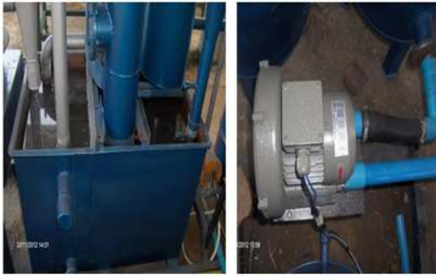
Figure 4. Heat exchanger and producer gas transmitter system.
