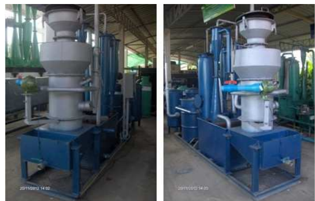
Figure 2. Producer gas Down Draft type.
