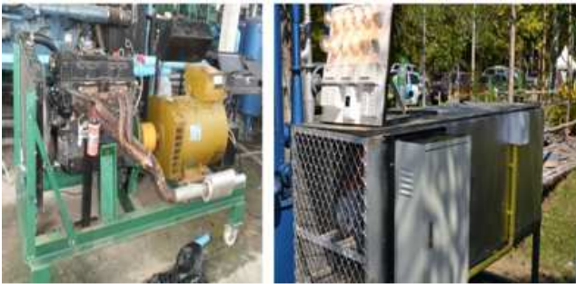
Figure 5. producer gas engine and load (heater).
