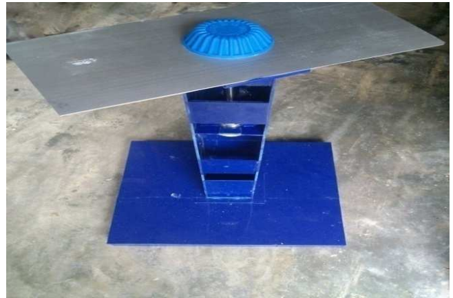
Fig. 9. Foundation of the solar tracker.
