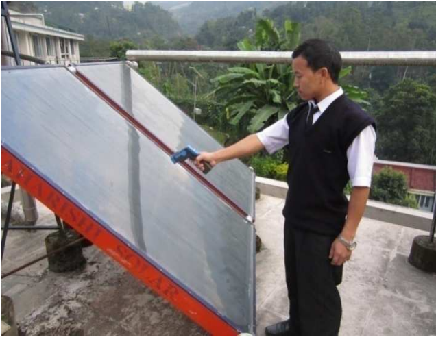
Figure 3. Measurement of surface temperature of solar collector
