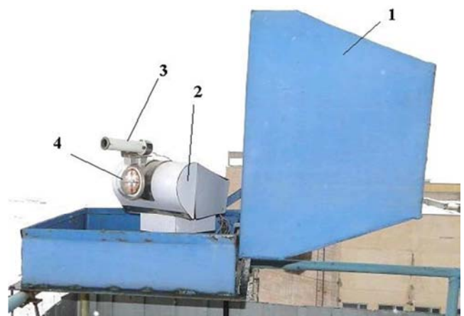
Figure 2. Shows the general view of the actinometric installation with a tracking system for the solar trajectory. The installation is located on the 6th floor of the BSF concentrator, near the laboratory room where the data is recorded (see Figure 2b).
